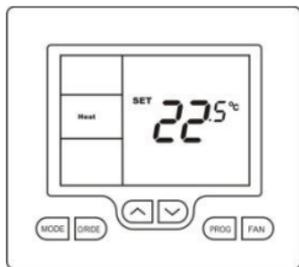
If Auto mode is selected, after adjusting the Heat set point wait without touching a button for 3 seconds for the thermostat display to change to show “Cool” and “SET” and your current cooling set temperature. If desired change this value with the up (▲) or down (▼) buttons. Again wait for three seconds to exit the temporary overridden programmed mode.
